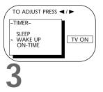
Press the PLAY/▲ button or the STOP/▼ button to select ON-TIME. Then, press the REW(ind)/◀ button or the F.FWD/▶ button to select your desired wake up time. Each press of the F.FWD/▶ button or the REW(ind)/◀ button will increase (or decrease) the time by 10 minutes.
